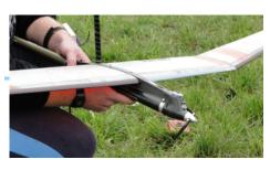
Nose of a power model (class F1C) with fully integrated motor
