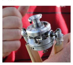
Propeller hub of rubber powered model
